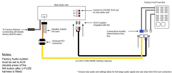
Ensure new audio unit settings allow for full range audio signal (not sub only) from RCA out connector
